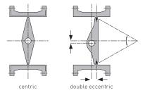
Another result of the double-eccentric design is reduced torque. Over time, traditional boot-style valves have a tendency to become harder to operate which is troublesome for maintenance and operation personnel. The increased torque can also cause electric actuators to fail prematurely. Even when comparing new valves, our design requires approximately 50% less torque.
