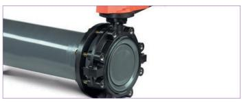
The 578 valve is designed to hold full pressure on either side of the valve while only one flange is present. This means one side of the system can be shut down for maintenance or expansion without having to depressurize the other side.
